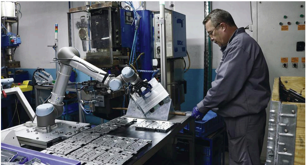
The robot must detect a case on a table with its camera, grip it, and put the case in the welding fixture. Then the robot goes for the front plate and puts it on the fixture. After that, the command is given for the machine to weld.
