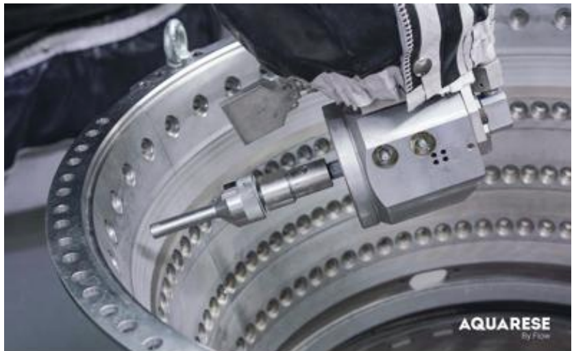
Waterjet cutters can be modified to handle stripping to remove coatings from turbine engine components used in jet engines. (Courtesy of Shape Technologies Group)
