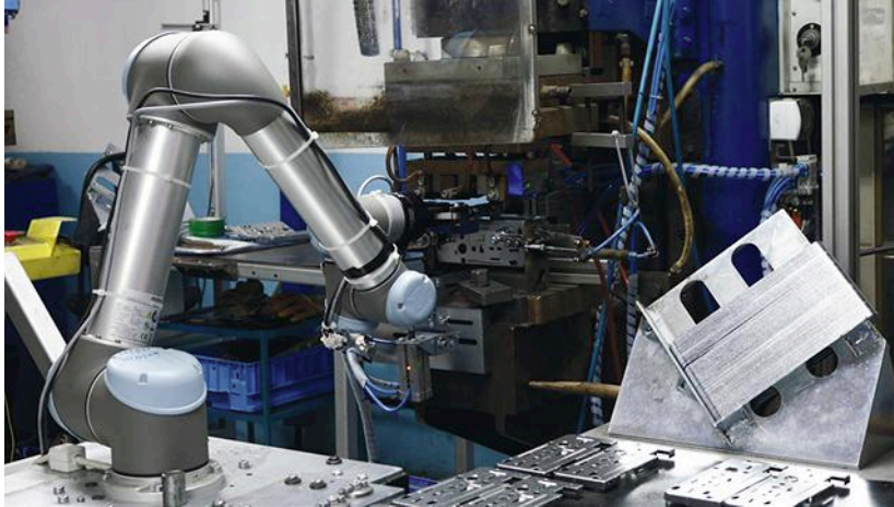
Cobots are able to load and unload parts to and from machines. In some factories there isn't enough space to have robots that require safety enclosures.
