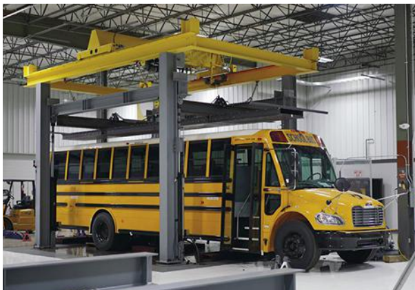
3. The vehicle roof-crush test system is operated by four hydraulic cylinders at the corners that must apply up to 100 tons of synchronized target force.
