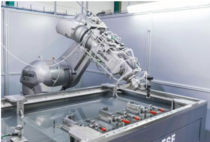
A robotic waterjet cutter from Shape Technologies Group uses supersonic water and garnet (an abrasive) to slice through and shape a variety of metals, including superalloys, used in the aerospace industry. (Courtesy of Shape Technologies Group)
