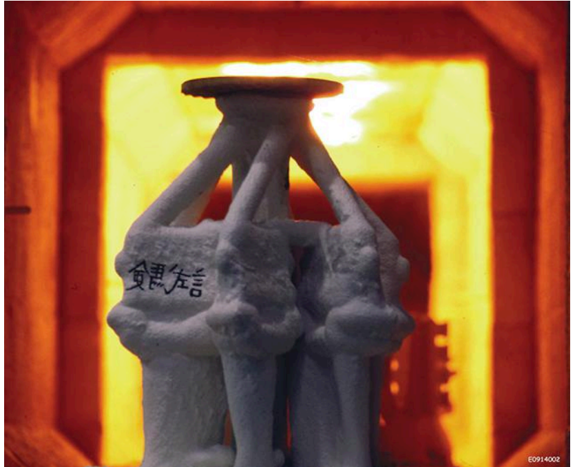
A ceramic mold created by repeatedly dipping wax molds of turbine blades into a ceramic slurry gets ready to go into the vacuum furnace at Howmet's Terai, Japan foundry. There it will be filled with molten superalloy to form directionally solidified turbine blades. (Photo courtesy of Howmet Corp.)
