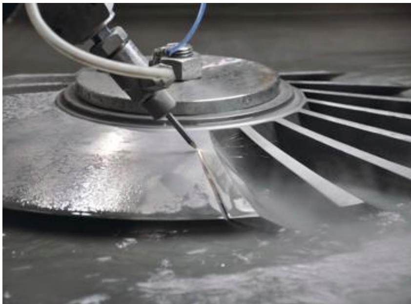
An abrasive waterjet controlled by a robot cuts a 3D part, a titanium blisk for a commercial jet engine. (Courtesy of Shape Technologies Group)
