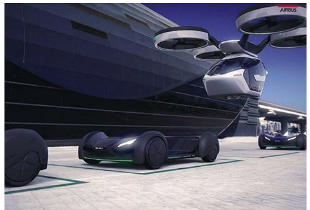
The main body of the car mounts to sleds which provide ground transportation. The rider can then request an air module from a nearby charging station to dock with the main body, which detaches from the sled for vertical liftoff.
