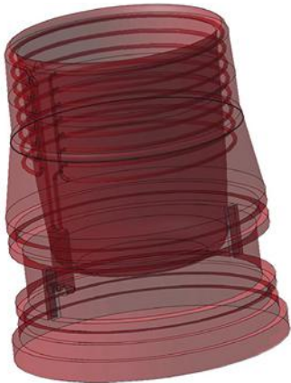
It took complex modeling software to determine the best architecture for internal, conformal cooling channels for this cylinder.
