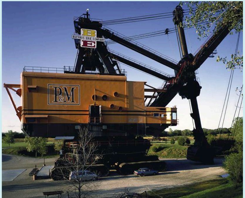
“Big Brutus” was the 11-million-lb. mine shovel used from 1963 to 1974 to move coal for the Pittsburg & Midway Coal Mining Co. in Kansas. Standing 160 feet tall, Big Brutus was a workhorse, averaging 5,000 cubic yards of coal per hour and able to dig in thick seams of coal. It was built by the Bucyrus-Erie Co., and worked with a bulldozer and two smaller shovels to extract and load coal, which was transported to regional power plants.
