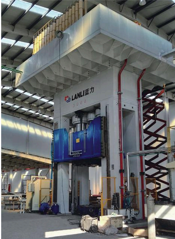
2. The platen in the automotive panel press must remain level even as up to 3,000 tons of force are being applied.
